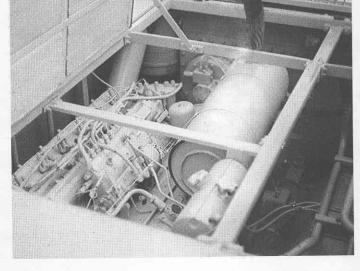
The engine with the special sound insulation offers a good accessibility to all components for easy maintenance.
